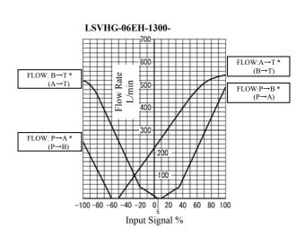
\* For "FLOW," the symbol outside parentheses represents the input signal type "A," "B," and "C"; the symbol in parentheses represents "D," "E," and "F."
