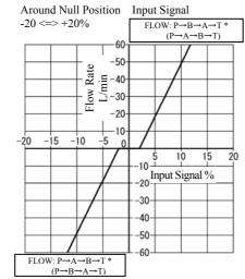
The load flow characteristics, step response, and frequency response are the same as those of the existing standard models.
