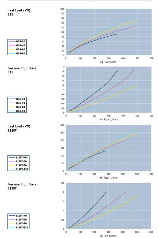
Inlet oil temperature 60°C at  $\Delta p$  max 2 bar Inlet water temperature 20°C
