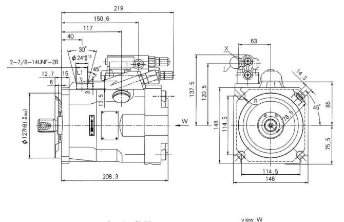
Port plate 61/11 shown is anticlockwiserotation For clockwise rotation, turn port plate 180°
